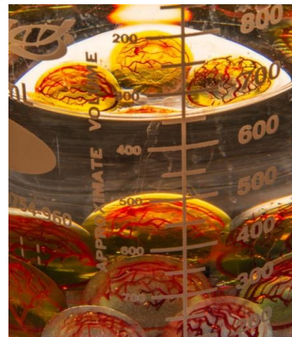
3D bioprinted soft tissue implant with vascularization channels printed with 3D Systems' SL bioprinter and BioInk that is based on CollPlant's rhCollagen.
