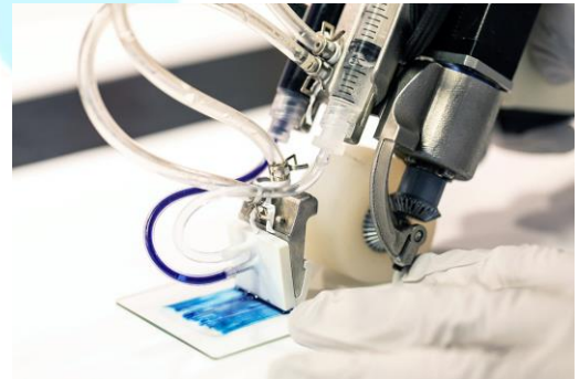
Handheld 3D skin printer developed at the University of Toronto; PHOTO: Daria Perevezentse)
